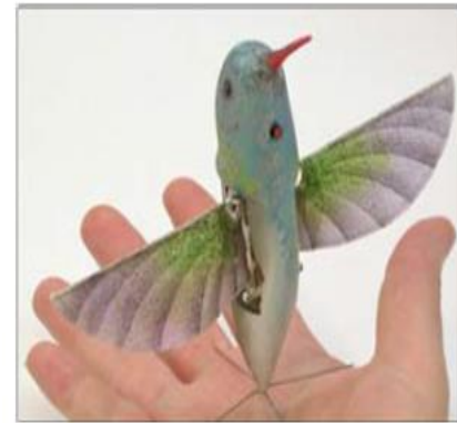
Nano Hummingbird by AeroVironment Inc. (Keennon et al., 2012) weight 19 g wingspan 16.5 cm endurance 4-11 min
